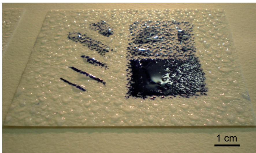
Fig. 2: Drops formed during ultrasonic mist treatment on Arches Aquarelle paper.
